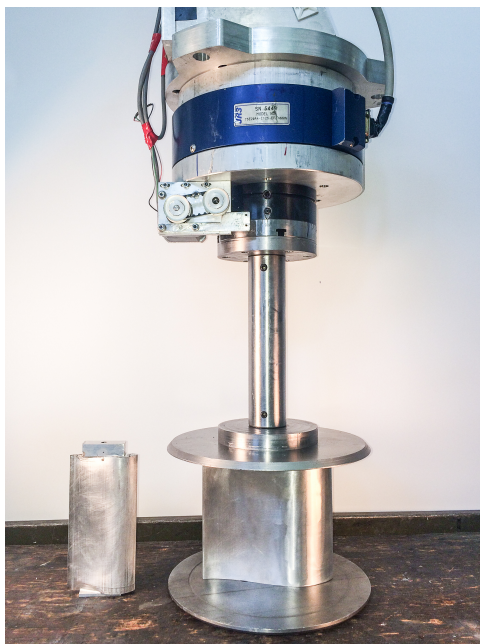
Figure 1. The experimental setup. From top to bottom: Mounting plate, force sensor in blue, rotary table with stepper motor, mounting rod, upper endplate, AR 1 - airfoil, lower endplate. AR 2 - airfoil for comparison on the left.
